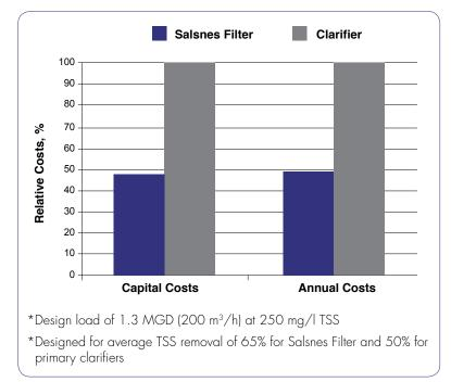
The above evaluation was completed by the Norwegian State Pollution Control Agency to discover cost efficient technology that could fulfill the European Union's stringent criteria for primary treatment. As you can see, savings are substantial. A Salsnes Filter system costs half that of conventional primary sedimentation and clarification.
