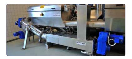
Separation, thickening and dewatering - all in one compact unit.
